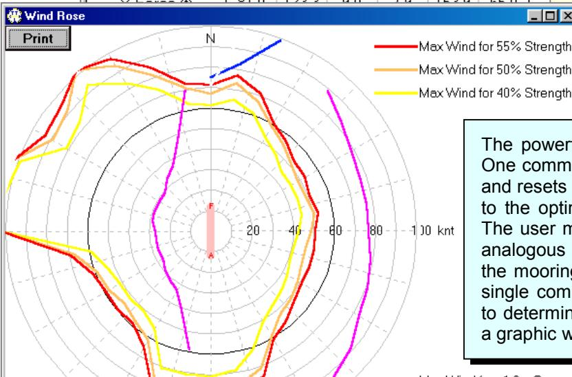
**OPTIMOOR** computes and displays vessel movements and mooring forces. Mooring line loads are shown in tonnes (or kips) and percent of rated breaking strength (RBS). Lines loaded to more than 55% of RBS are highlighted in red. The analysis results are also reflected on the plan graphic display and the numeric results can be printed out.
